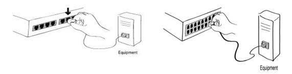
Figure 2-6 Connecting a equipment to the STS400/800(Left) / STS1600(Right)
