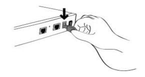
Figure 2-3 Connecting the power to the STS400/800
