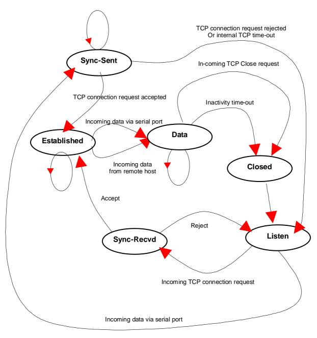
Figure 4-6 State Transition Diagram of TCP mode
