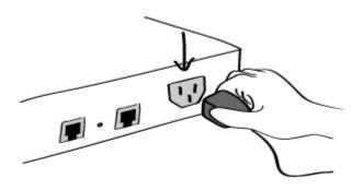
Figure 2-4 Connecting the power to the STS1600
