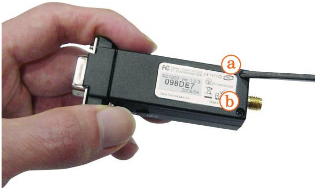
Figure 2-5 Remove Parani-SD1000 bottom cover
