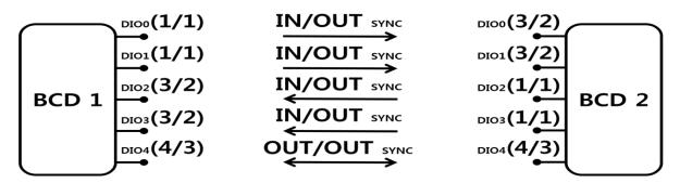
Figure 5-2 DIO Synchronization According to I/O Configuration and DIO Synchronization Configuration
