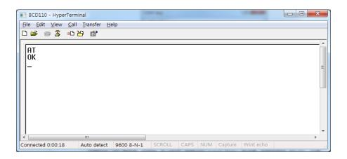
Figure 2-6 Testing AT Command on HyperTerminal
