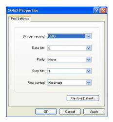
Figure 2-5 HyperTerminal Serial Setting
