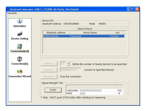
Figure 3-7 Signal Strength Test
