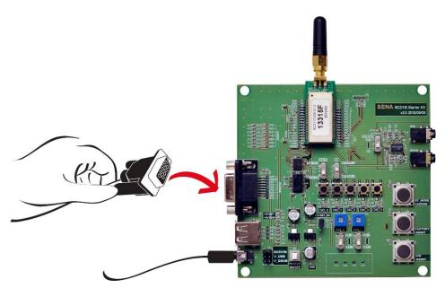
Figure 2-4 Connecting a Device to Development Board
