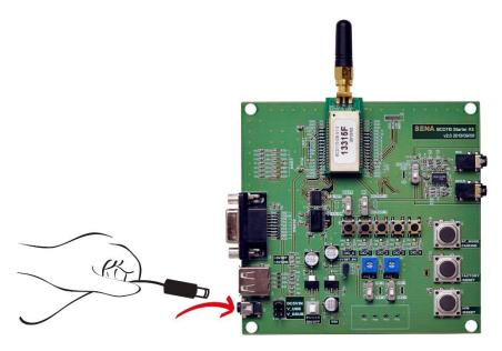
Figure 2-3 Connecting Power to Development Board
