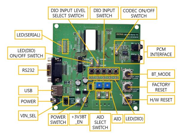
Figure 2-1 The Panel Layout of BCD Development Board
