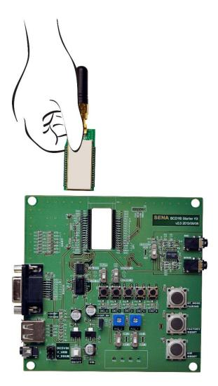
Figure 2-2 Connecting Parani-BCD110 to Development Board
