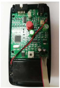
The STATUS line is marked by the red wire on the ribbon cable in this picture.
