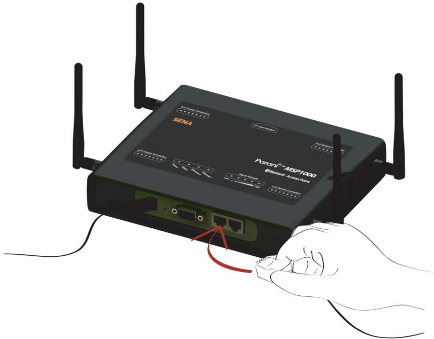
Figure 2-3 Connecting a network cable to the Parani-MSP1000
