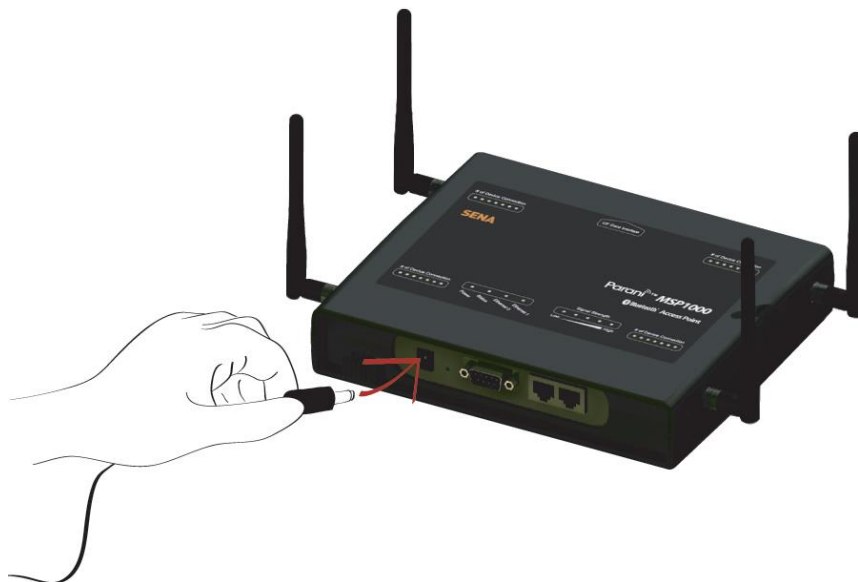
Figure 2-2 Connecting the power to the Parani-MSP1000
