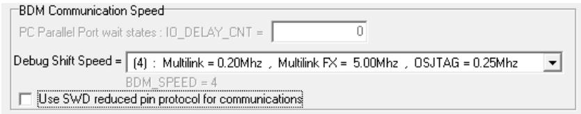
**Figure 5-8: Clear Checkbox To Use JTAG Communications Mode**
