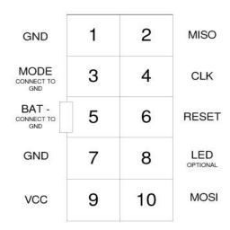
TOP VIEW OF THE CONNECTOR ON THE PROGRAMMER
